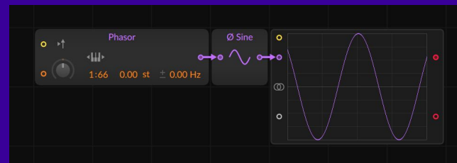
Generating sine wave using phase generator
